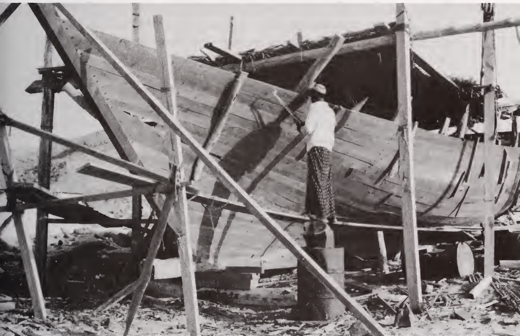
Ar Rustaq fort, Oman, restored by Omani Ministry of National Heritage and Culture Building a dhow in Sur, Oman's ancient port; ship construction is a major enterprise of Persian Gulf states. Courtesy Embassy of the Sultanate of Oman, Washington
